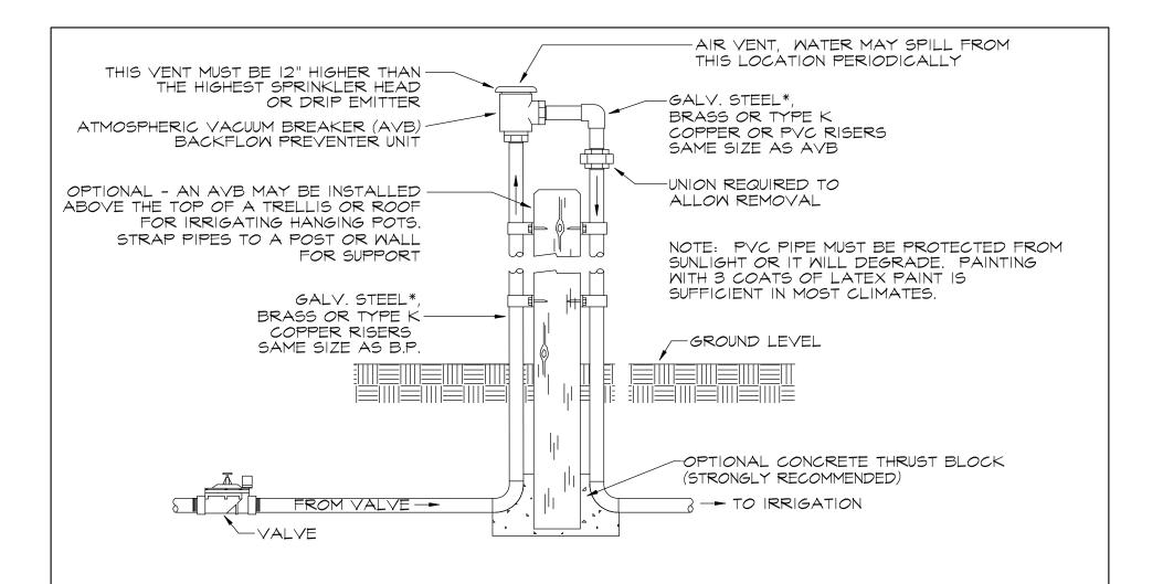
WRAP ENTIRE ASSEMBLY WITH INSULATION TAPE FOR LIGHT FREEZE PROTECTION. DO NOT BLOCK AIR VENT ON BACKFLOW PREVENTER,
