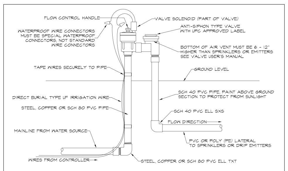
VALVE WILL FAIL EARLY IF VALVE WIRE CONNECTIONS ARE NOT COMPLETELY WATER PROOF. INSTALL WIRE UNDER MAINLINE TO PROTECT IT.
